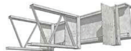
12. HJ SMALLER BEAM WITH VERTICAL SHS STUBS WELDED TO FLANGES BY HOPLEYS OR STEEL FABRICATOR
