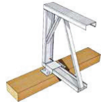
5. HJ TO WALLPLATE USING NAIL CLIP (END-CLIP WELDED BY HOPLEYS)
